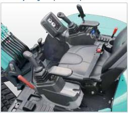
The new redesigned operators station includes such features as a newly designed monitor, 2 speed travel switch located on the backfill blade lever, and the auxiliary hydraulic switch located on the joystick.
