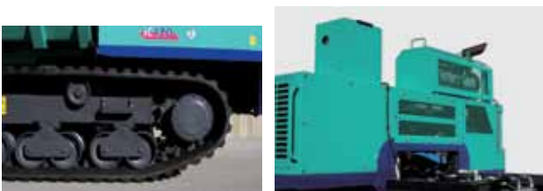
Maintenance is made easy with segmented sprockets, all travel motors and lowers rollers are sealed. Rear engine covers are removeable to easily access components such as hydraulic valves, solenoids, and the engine filtering systems.
